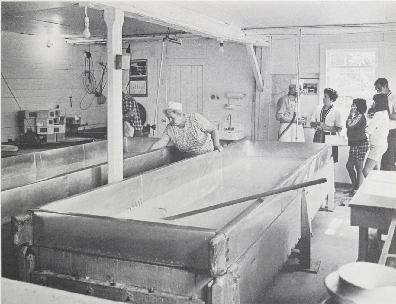
The process starts with 3,500 to 4,000 pounds of whole milk gradually warmed from forty degrees. Curd is formed in about an hour.
