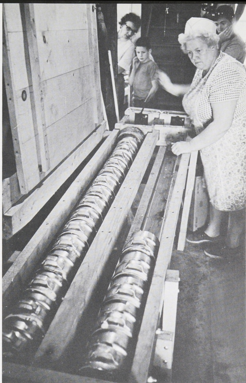
Set end-to-end, the hoops are pressed to squeeze out all the whey.
